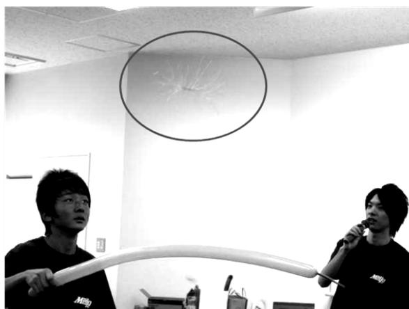
**FIGURE 1.** “Angel hair” is flowing up against gravity because of the repulsive force between the “angel hair” and the pencil balloon.
