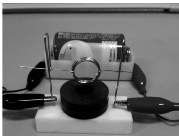
**FIGURE 3.** “Motor” made from paper clip and other things easy to get.
